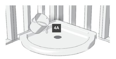
If water doesn't drain properly even though the base is leveled, do not continue this installation. Please remove the base and return it to your dealer for
