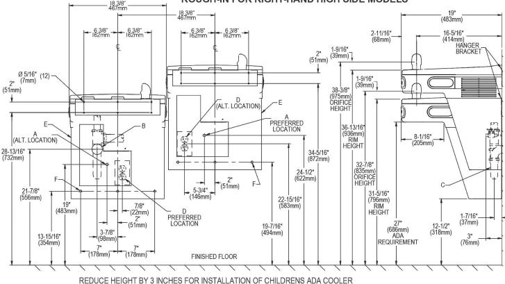
LEGEND A = Recommended water supply location. Shut off valve (not furnished) to accept 3/8" O.D. unplated copper tube connect. Up to 3" (76mm) maximum out from wall.
