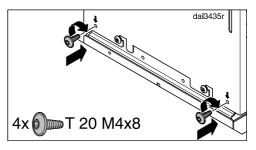
Secure the hood with the screws supplied.
