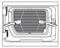
■ Push the plinth filter in completely.
