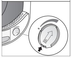
■ To open the cover, push the tab all the way up to the top.
