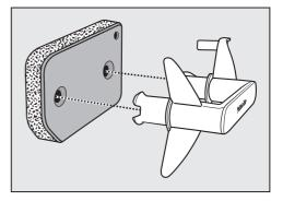
Install the plinth filter back on the handle. Make sure it is the correct way round.
