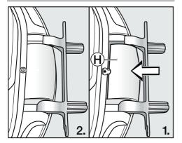
■ Fit new door hinge cover (H) and clip it into position.
