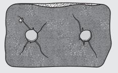
Lint will blow into the heat exchanger through cracks and tears. This will cause a permanent obstruction in the heat exchanger. White residues or residues of other colors
