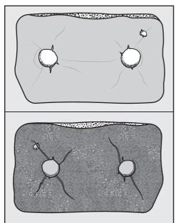
Lint will blow into the heat exchanger through cracks and tears. This will cause a permanent obstruction in the heat exchanger. White residues or residues of other colors
