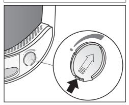
If you are not using a fragrance flacon: Push the tab down completely (see arrow) to close the socket. Otherwise, lint will accumulate here.
