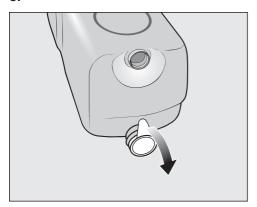
Remove the film seal from the cartridge completely. Risk of damage from film seal If the film seal is not removed completely, leaks can occur in the TwinDos system.
