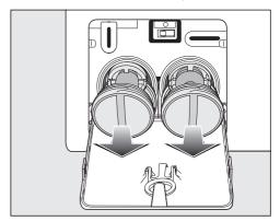
■ Remove the drain filters completely.
