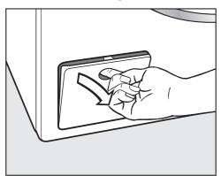
■ Open the drain pump flap.
