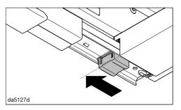
Slide the depth stops forward to the position shown.
