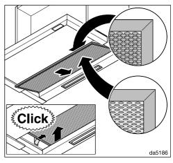
■ Reinsert the grease filter.
