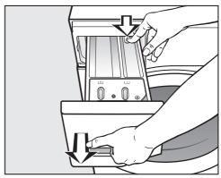
■ Pull out the detergent dispenser drawer until a resistance is felt. Press down the release button and at the same time pull the drawer right out of the machine
