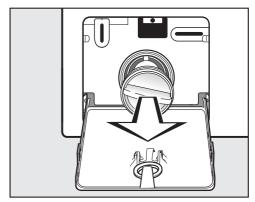
■ Remove the drain filter completely.
