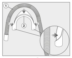
■ Attach the elbow ② to the drain hose ①.
