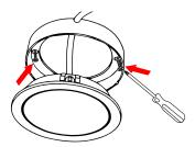
3. Secure housing to mounting surface with 2 screws, included.
