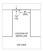
ICE MAKER DRAIN Ice maker models can be ordered with or without a drain pump. Models without a pump will drain water by gravity. A drain must be provided for all models
