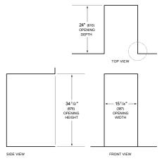
NOTE: 31/2" (89) finished returns will be visible and should be finished to match cabin
