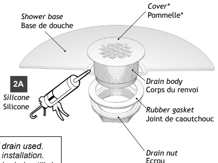
Components might vary according to the model of drain used. Refer to manufacturer's instructions for the proper installation.
